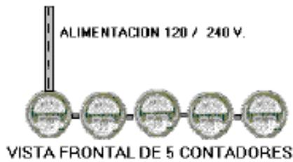
**MEDICION EN BAJA TENSION 120/ 240 V. CON ACOPLAMIENTO DE 5
